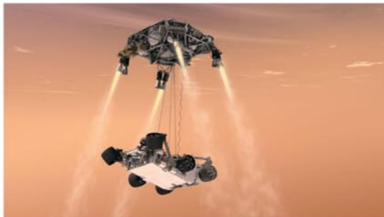
3 Rockets slow spacecraft to halt; "sky crane" tether lowers rover to surface.
