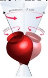
Earth's axis precesses like the axis of a spinning top.
