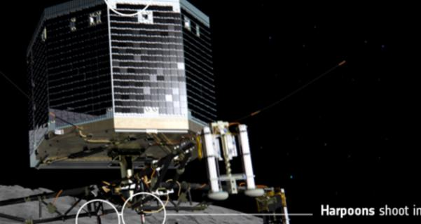
Foot screw starts drilling upon impact with the surface
